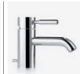
33 501 625 / 33 526 625 / 33 551 625* / 33 556 625* Single-lever basin mixer with/without pop-up waste, 125 mm projection Miscelatore monocomando lavabo con/senza piletta, sporgenza 125 mm Monomando de lavabo con/sin válvula automática, saliente 125 mm [7 l/min.]
