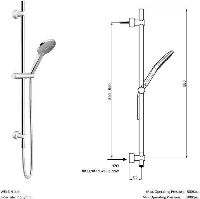
Min. Operating Pressure: 100Kpa. Pipework must be flushed before installation Please install as per manufacturers instructions in the box
